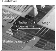
Flexures and electrostatic actuators
